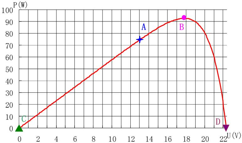
Figure3-2 Voltage-Power Curve
